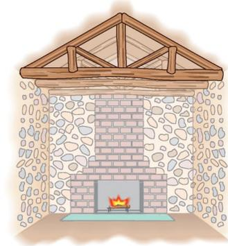
FIGURE 12-26 A roof truss.
