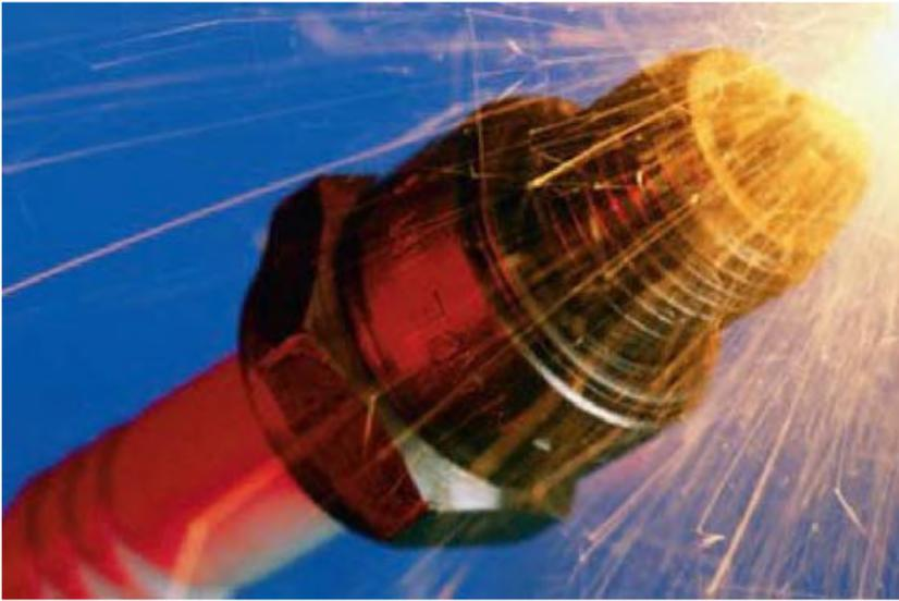
A spark plug in a car receives a high voltage, which produces a high enough electric field in the air across its gap to pull electrons off the atoms in the air–gasoline mixture and form a spark. The high voltage is produced, from the basic 12 V of the car battery, by an induction coil which is basically a transformer or mutual inductance. Any coil of wire has a self-inductance, and a changing current in it causes an emf to be induced. Such inductors are useful in many circuits.
