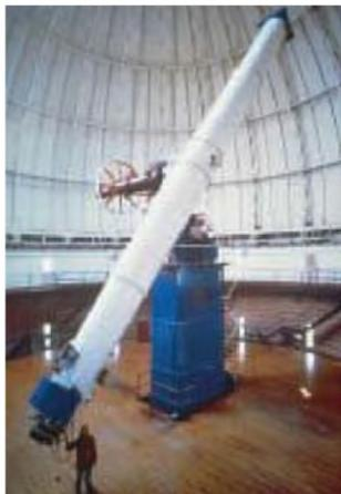
**EXAMPLE 33–15 Telescope magnification.** The largest optical refracting telescope in the world is located at the Yerkes Observatory in Wisconsin, Fig. 33–37. It is referred to as a “40-inch” telescope, meaning that the diameter of the objective is 40 in., or 102 cm. The objective lens has a focal length of 19 m, and the eyepiece has a focal length of 10 cm. (a) Calculate the total magnifying power of this telescope. (b) Estimate the length of the telescope.
