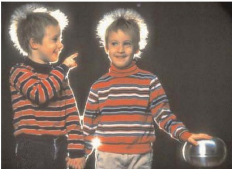
We are used to voltage in our lives—a 12-volt car battery, 110 V or 220 V at home, 1.5 volt flashlight batteries, and so on. Here we see a Van de Graaff generator, whose voltage may reach 50,000 V or more. Voltage is the same as electric potential difference between two points. Electric potential is defined as the potential energy per unit charge.
