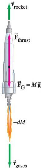
**FIGURE 9-35** Example 9-20;  $\vec{v}_{\text{rel}} = \vec{v}_{\text{gases}} - \vec{v}_{\text{rocket}}$ .  $M$  is the mass of the rocket at any instant and is decreasing until burnout.
