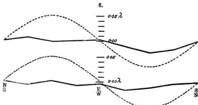
placement due to the relative motion of the earth and the luminiferous ether, this cannot be much greater than 0·01 of the distance between the fringes.
