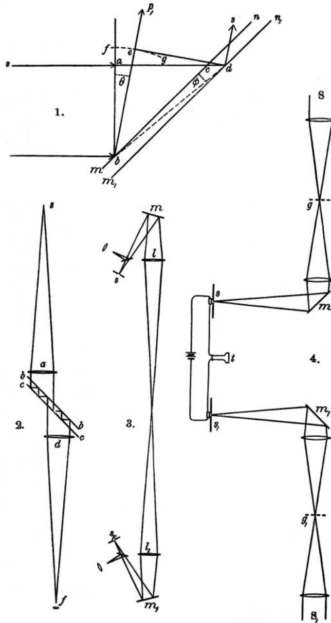
would be about one-millionth of the original intensity, so that if sunlight or the electric arc were used it could still be readily seen. The mirrors *bb*, and *cc*, would differ from parallelism sufficiently to separate the successive images. Finally, the apparatus need not be mounted so as to revolve, as the earth's rotation would be sufficient.
