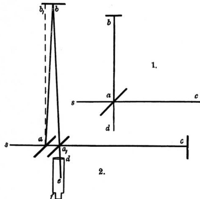
and  $ca$  is partly reflected along  $ad$ . If then the paths  $ab$  and  $ac$  are equal, the two rays interfere along  $ad$ . Suppose now, the ether being at rest, that the whole apparatus moves in the direction  $sc$ , with the velocity of the earth in its orbit, the direc-
